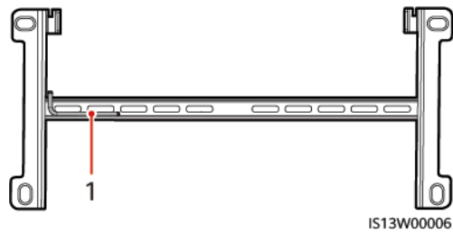
Figure 4-9 Position for binding the security Torx wrench.
