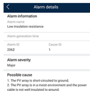
Figure E-1 Alarm details
