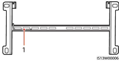
Figure 4-9 Position for binding the security Torx wrench.
